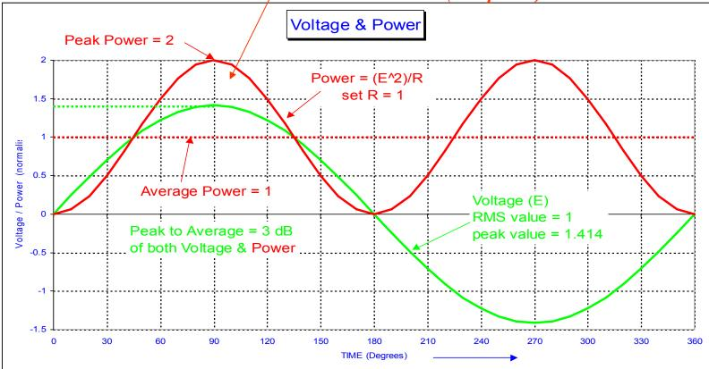
The RMS voltage equals the equivalent DC voltage required to provide the same heating or average power when applied to a resistive load.
